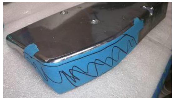
Figure 3. Sharpie marks indicating cutting zone for license plate holder and pipe clearance ( NOTE: Your fitment and trimming may be different than shown in the picture).
