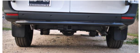
Figure 3: Hitch Clearance with Rear Nerf Step Installed
