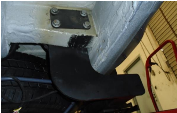
Figure 2: Four (4) of the Hitch Mounting Bolts
