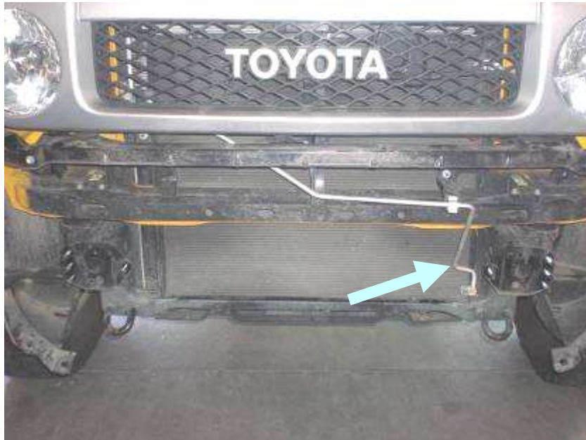
Figure 5: Air conditioning refrigerant tube
